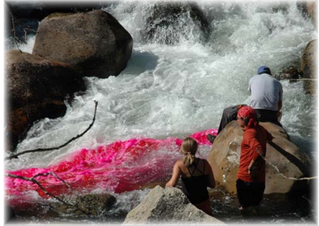
Water scientists use trace dye to understand stream flow patterns.
