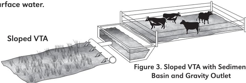
Figure 3. Sloped VTA with Sediment Basin and Gravity Outlet
