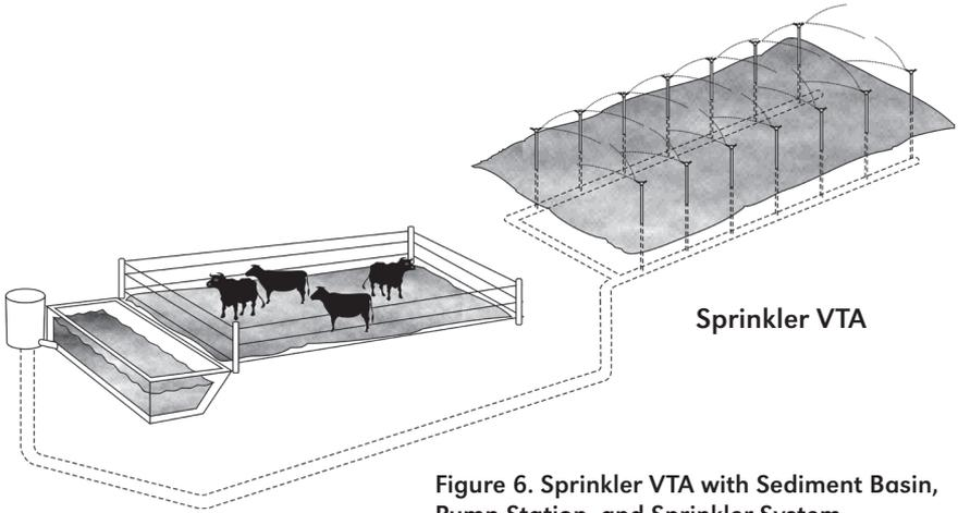
Figure 6. Sprinkler VTA with Sediment Basin, Pump Station, and Sprinkler System
