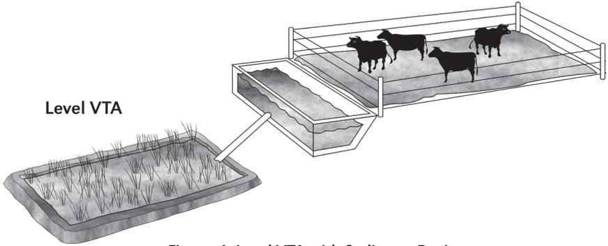
Figure 4. Level VTA with Sediment Basin
