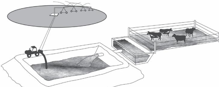
Figure 1. Conventional Holding Pond Runoff Storage System
