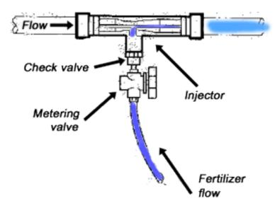
Figure 3. Schematic drawing of a venturi injector.
