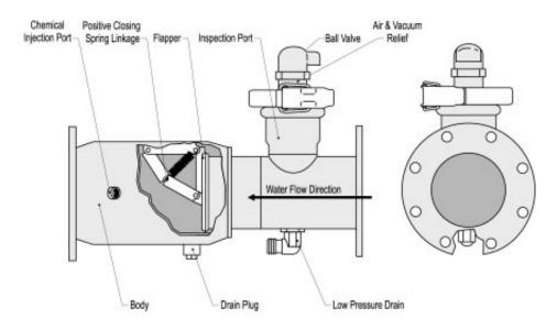
Figure 4. Schematic drawing of typical irrigation pipeline check valve.
