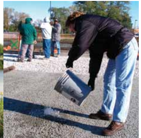
Pervious concrete allows water to quickly infiltrate the surface and subsurface layers while providing the structural soundness of a paved surface.
