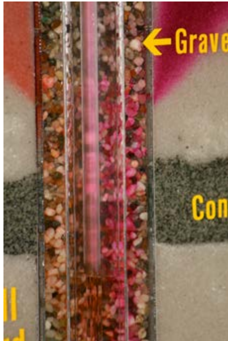
Figure 9. Dye Traveling Down Gravel Packed Annulus
